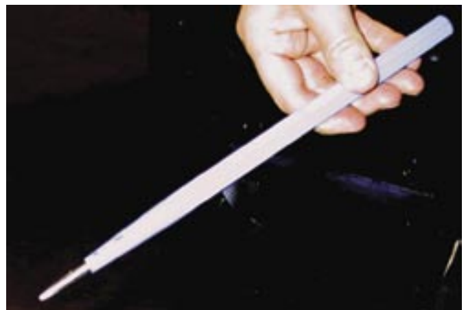
Figure 30. 0.25" (6.35 mm) drift punch
